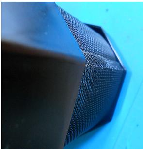
I roll it so that it is a little over wound, insert, encourage it to relax so the start and end align, then remove, re-centre the start, then reinsert.
