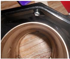
Insert 4gx12 self tappers in lower. Squeeze up the unit before tightening each screw.
